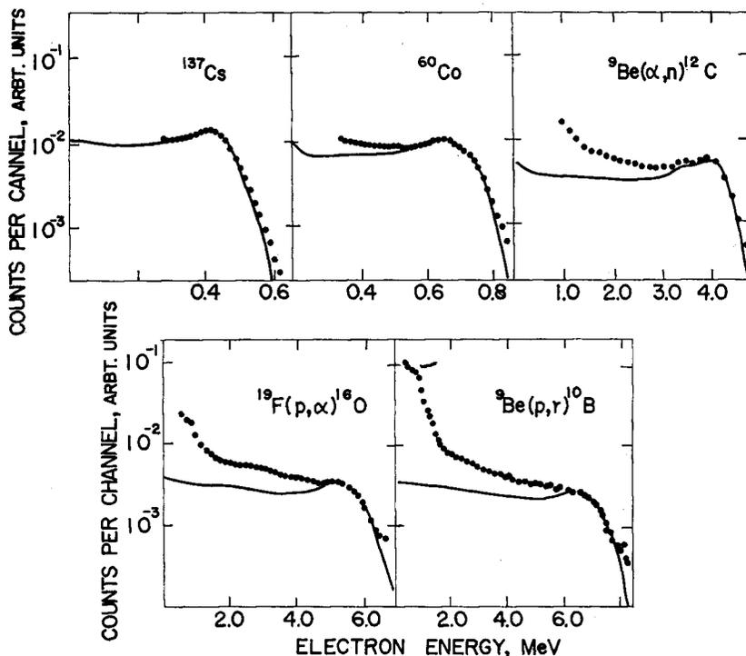
Fig. 2. Pulse height distributions obtained by a liquid Scintillator for gamma rays from  $^{137}\text{Cs}$  (0.662 MeV),  $^{60}\text{Co}$  (1.172 and 1.333 MeV),  $^9\text{Be}(\alpha, n)^{12}\text{C}$  (4.43 MeV),  $^{19}\text{F}(p, \alpha)^{16}\text{O}$  (6.13 MeV) and  $^9\text{Be}(p, r)^{10}\text{B}$  (7.48 MeV)—dots. Curves are shown calculated value.
