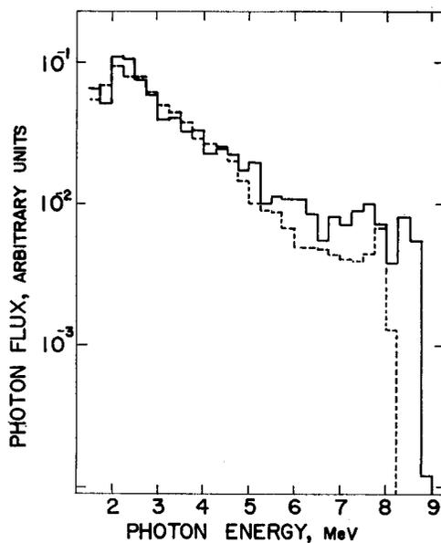
Fig. 7. Spectrum of gamma rays from the reactor core of "Yayoi" and passing through iron barrier of 15 cm in thickness (solid line). Estimated spectrum considering the attenuation in the iron barrier for gamma rays shown in Fig. 6 (dotted line).
