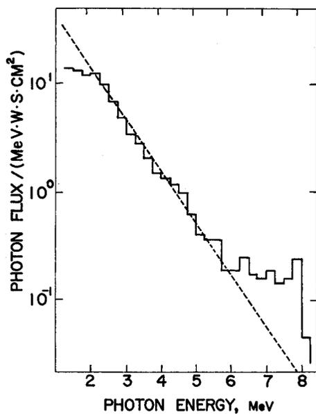
Fig. 6. Energy spectrum of gamma rays from the Fast Neutron Source Reactor "Yayoi" and Semi-Empirical formula for fission gamma rays obtained by Goldstein<sup>18)</sup>.
