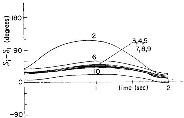
Fig. 9. The swing curves for the 10-machine system; heavy loads, fault 11-12 cleared at 0.06 sec.
