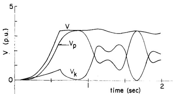
Fig. 7. The time variations of the Lyapunov function and its components for the 4-machine system; fault 2-1.
