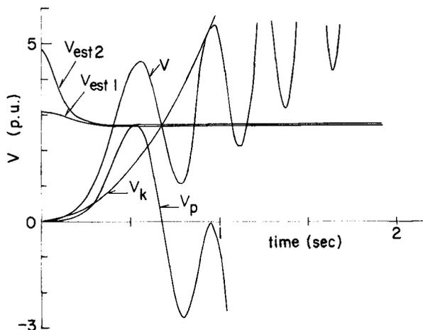
Fig. 5. The time variations of  $V_{est1}$  and  $V_{est2}$  for the 4-machine system; fault 3-4.
