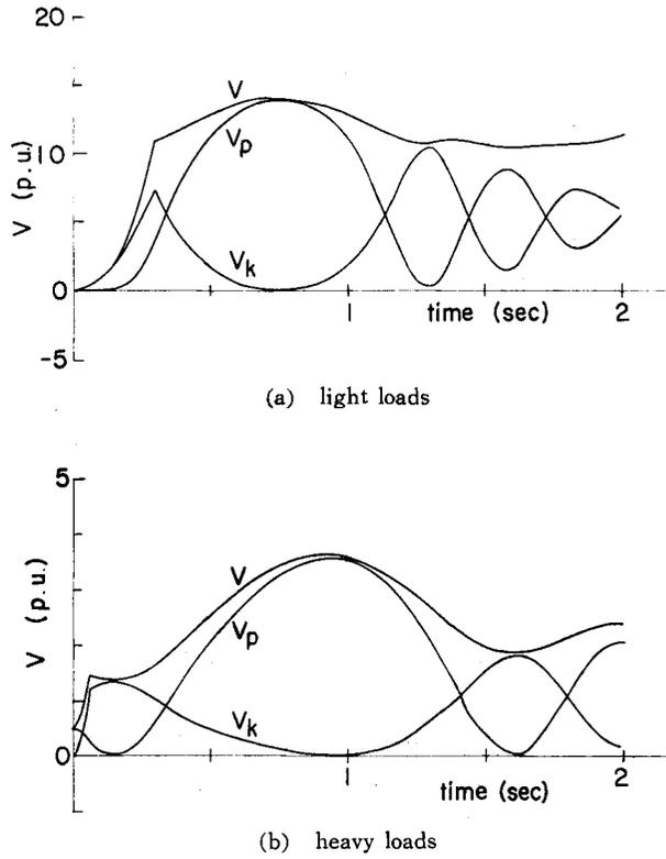
Fig. 8. The time variations of the Lyapunov function and its components for the 10-machine system; fault 11-12.
