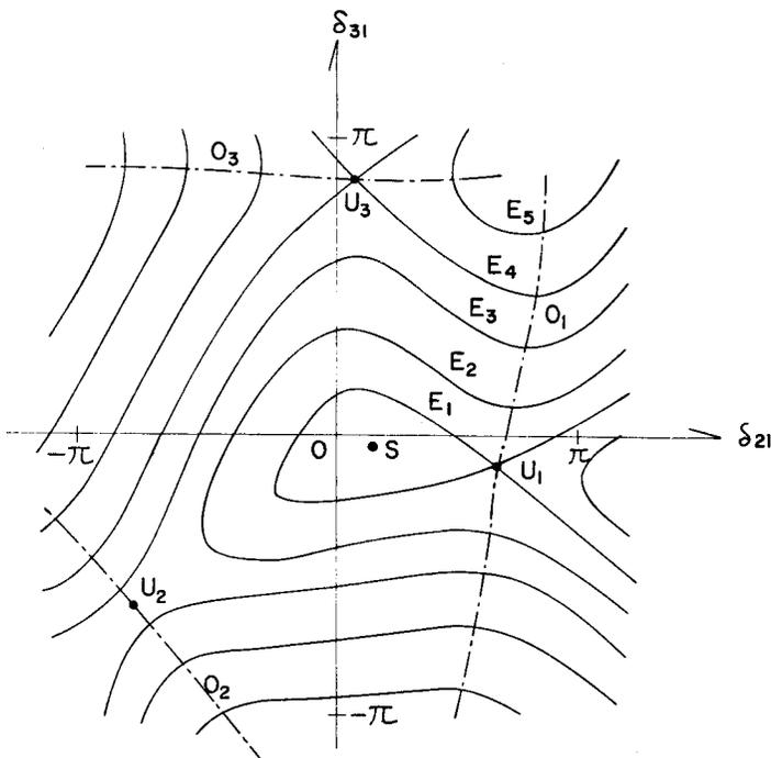
Fig. 2. Equipotential curves for a 3-machine system.
