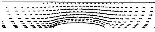
Fig. 8-2. Velocity vectors for a case with R=40 . The H -type grid is used.
