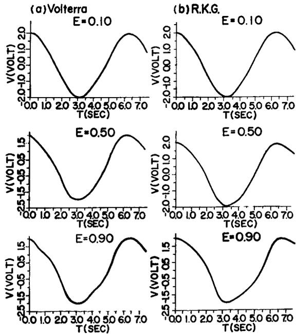
Fig. 7 Steady state oscillation wave of van der Pole oscillator
