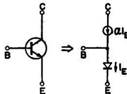
Fig. 11 Equivalent model of transistor
