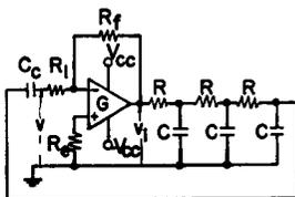
Fig. 8 CR low pass phase shift oscillator
