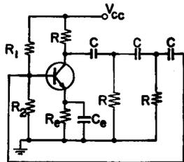
Fig. 10 Transistor CR phase shift oscillator
