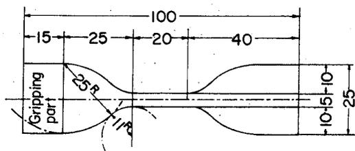
Fig. 1 Specimen of dumb-bell shape No. 3
