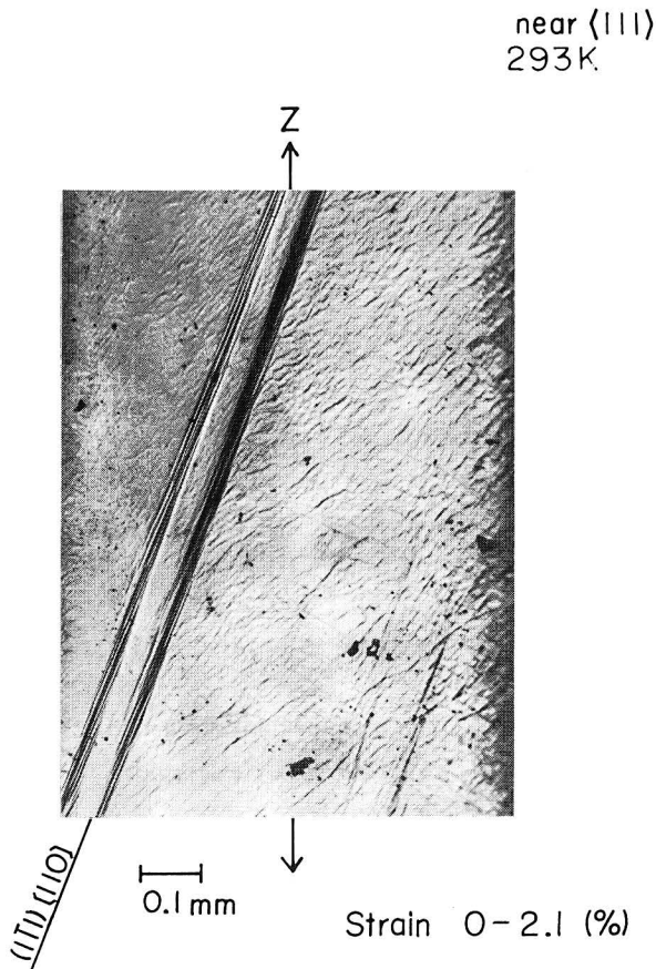
Fig. 8 Clustered slips observed in a near \langle 111 \rangle oriented single crystal stretched by 2.1% at 293 K.
