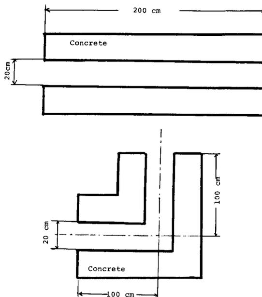
Fig.1 Concrete duct arrangements for the test calculation.
