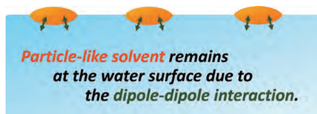
Figure 3. Schematic image of fluorinated solvents remaining on the water surface.
