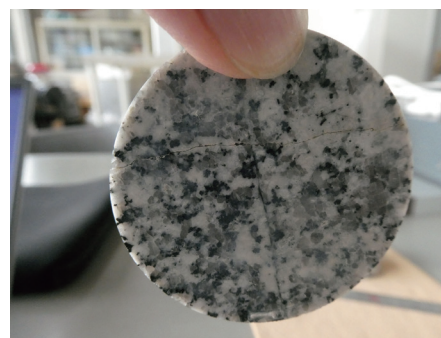
Fig. 14 Photograph of specimen TG-f2 after permeability measurement using water including clays. The macro-fracture is closed by the accumulation of clays.
