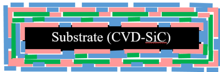
Figure 6.19 The schematic diagram of coating by multi-dipping on the substrate (Colors indicate different dipping times).
