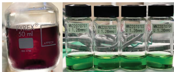
Fig. 1. Prepared U solution; (a) U(III) and (b) U(IV) in HCl solution.
