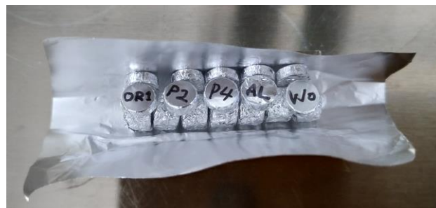
Fig. 1. Meteorite samples and mineral standards in the sapphire containers wrapped with Al foils.
