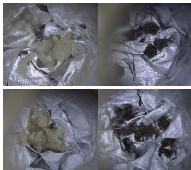
Fig. 2. Irradiated meteorite plagioclase (left column) and pyroxene (right column) samples in the Al foil capsules. The width of each photo is approximately 1 mm.
