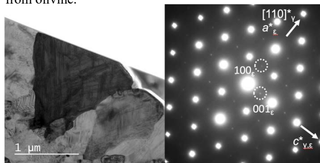
Fig. 2. Transmission electron micrograph (Left) and selected-area electron diffraction pattern (Right) of a ringwoodite ( \gamma ) grain with intergrown poirierite ( \epsilon ).
