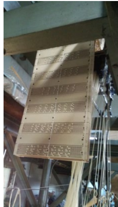
Jacquard machines and punch cards Taken at Fukuoka Weaving in Kyoto
