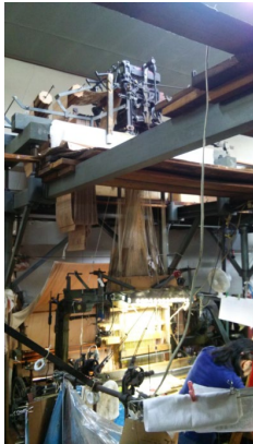
Jacquard machines and punch cards Taken at Fukuoka Weaving in Kyoto
