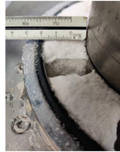
(c) A photo of an experimental shear zone in fine halite particles (thin)
