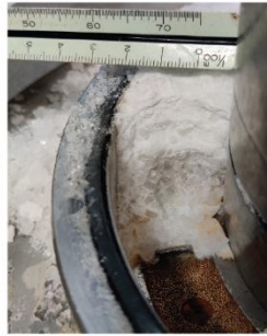
(b) A photo of an experimental shear zone in coarse halite particles (thick)
