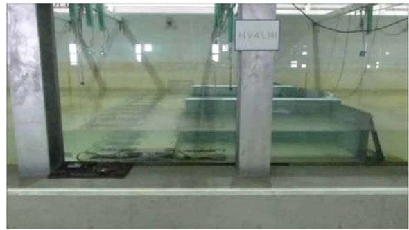
Photo 15 Experiment for effect of Fin-type movable breakwater to reduce tsunami force acting on visor gate
