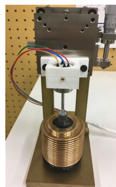
Photo 4 The self-recording aneroid barometer after improvement
