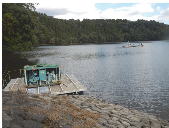
Fig. 3. The shot point in 2022 in far side and the high-pressure air compressor in near side
