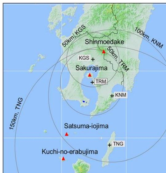
Fig. 1 Target volcanoes and operational weather radars in the South Kyushu region. The locations of the volcanoes and the weather radars are shown by triangles and plus signs, respectively. KSG: C-band Doppler radar at Kagoshima airport, TRM: X-band polarimetric radar at Tarumizu, KNM: C-band polarimetric radar at Kunimiyama, and TNG: C-band polarimetric radar at Tanegashima. Circles show the quantitative observation area of each radar.
