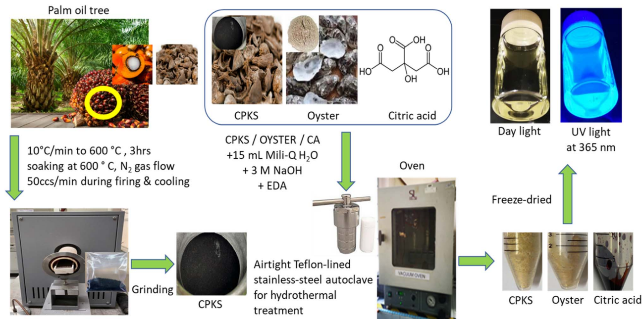
Fig. 1 Carbon QDs synthesis steps from CPKS, oyster shells, and citric acid sources.
