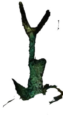
Fig. 6. An approximated surface mesh obtained by AlphaShape. Image captured by Meshlab application.
