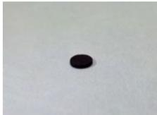
Figure 4 Porous MoO<sub>2</sub> pellet was produced
