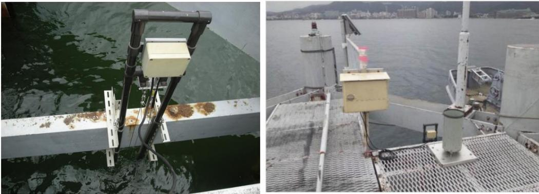
Figure 2 – 2. Photographs of the water level gauge (left) and observation site (right) with rain and water level gauges deployed at the Yanagasaki pier.
