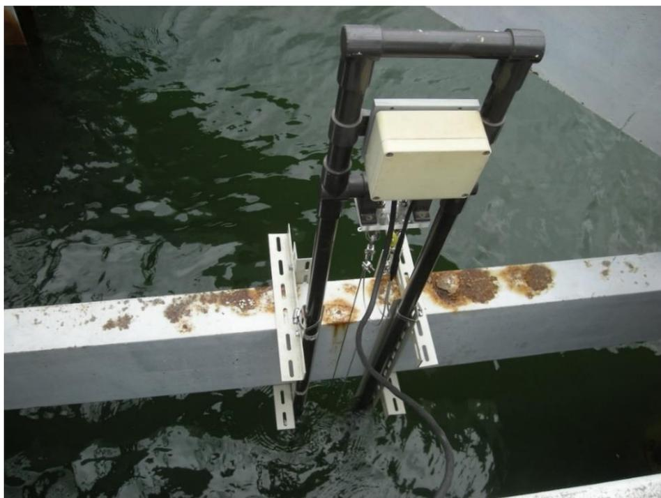
Figure 3 – 3. Capacitance type water level instrument.
