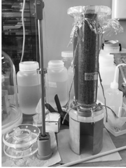
Setting up the column leaching tests: (a) After compaction, and (b) During permeation.
