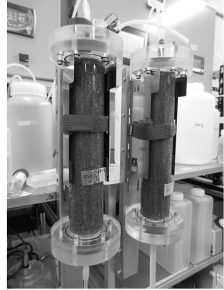
Setting up the column leaching tests: (a) After compaction, and (b) During permeation.
