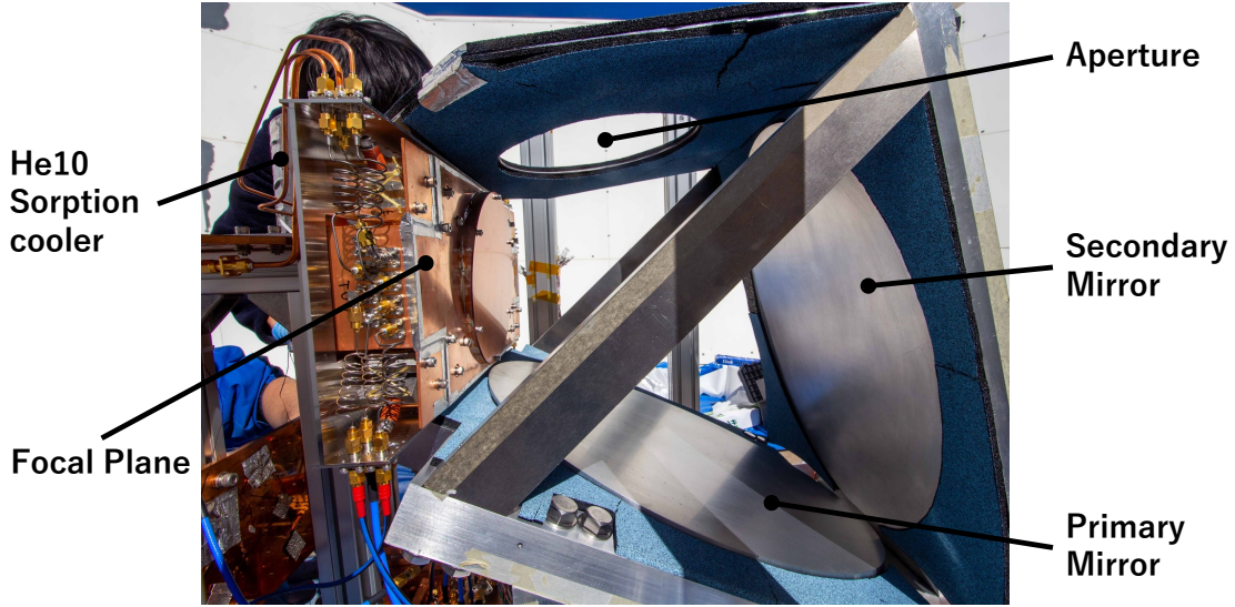
Figure 2.6: Picture inside the cryostat. The surface except the mirrors is covered by the absorber. We use Mizuguchi–Dragnone dual reflector which is a combination of a primary paraboloid and a secondary hyperboloid mirror.
