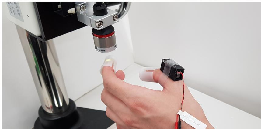
FIGURE 2.7: Overview of the experimental setup to measure the noise at a finger.
