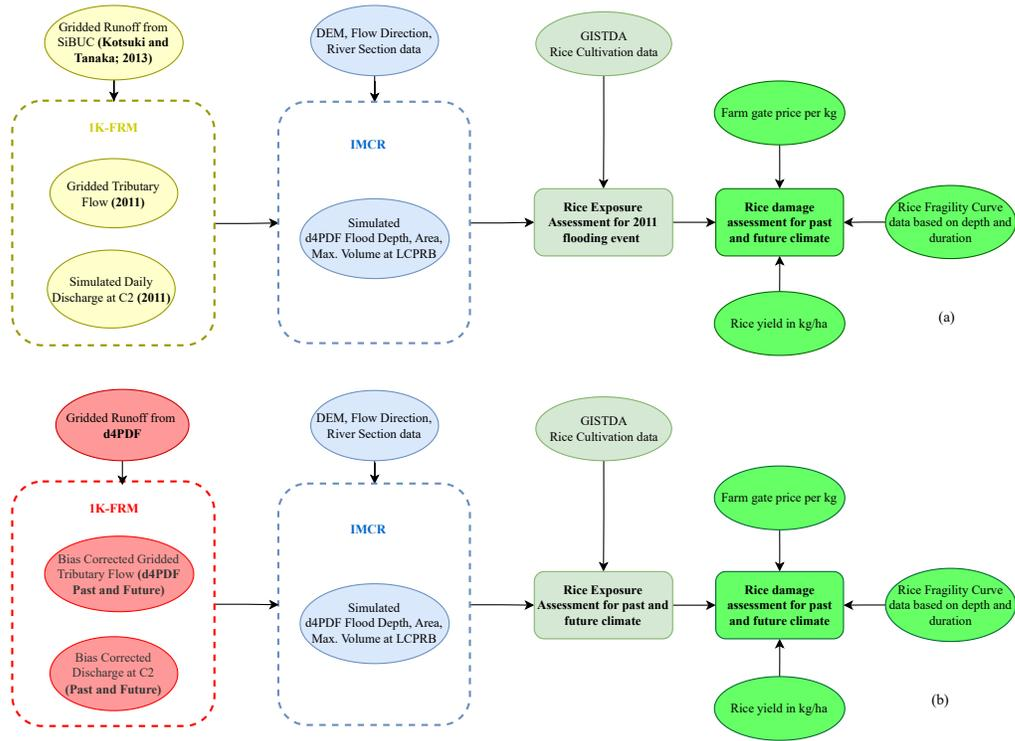
Figure 6.1: Methodological framework opted for the agriculture damage assessment for (a) 2011 flood as model validation and (b) d4PDF past and future climate in the LCPRB.
