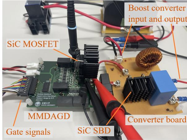
Figure 5.6: Photograph of boost converter with MMDAGD.
