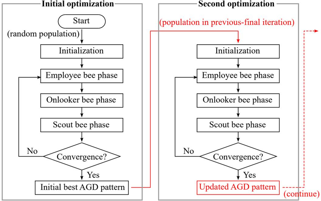
Figure 5.2: Flowchart of ABC-algorithm-based optimization and updating scheme for MMDAGD in continuous operation.
