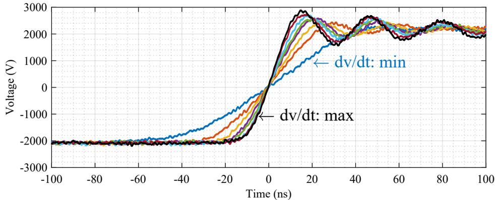
Figure 1.4: Example of output voltage waveforms of SiC MOSFET full-bridge with different values of  $R_G$  ranging from  $5\ \Omega$  ( $dv/dt$ : maximum) to  $40\ \Omega$  ( $dv/dt$ : minimum).
