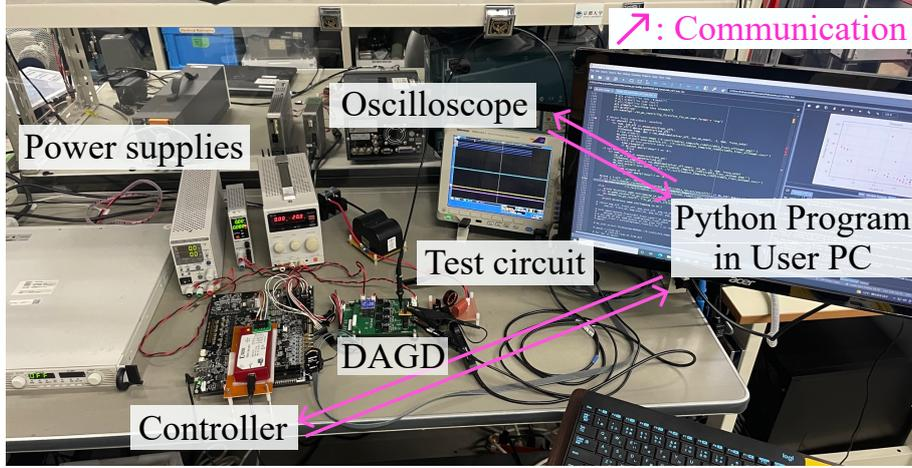
Figure 3.7: Photograph of laboratory experiment setup. © 2023 IEEE.
