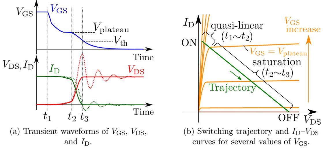
Figure 2.2: Examples of switching waveforms of MOSFET during turn-off, assuming load is an ideal resistor.
