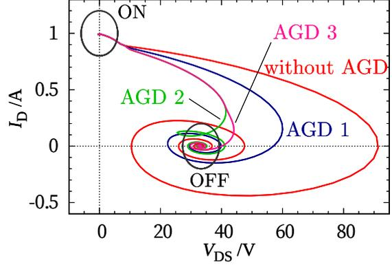
Figure 2.13: Simulated switching trajectories without/with AGD.
