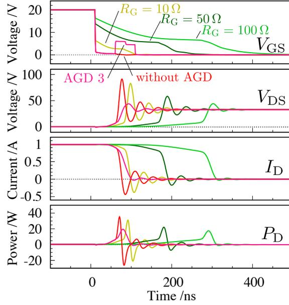
Figure 2.14: Simulated switching waveforms without AGD, with AGD 3, and with CGD ( $R_G = 10/50/100 \Omega$ ).
