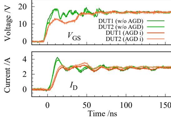
Figure 4.8: Turn-on switching waveforms in case 1 with AGD and without AGD. AGD i: 0x0 → 0xA (40 ns) → 0xF. © 2023 IEEE.
