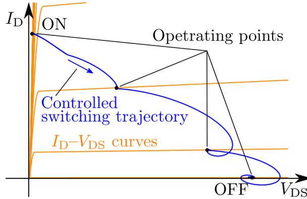
Figure 2.3: Conceptual diagram of switching trajectory control using discrete operating points.
