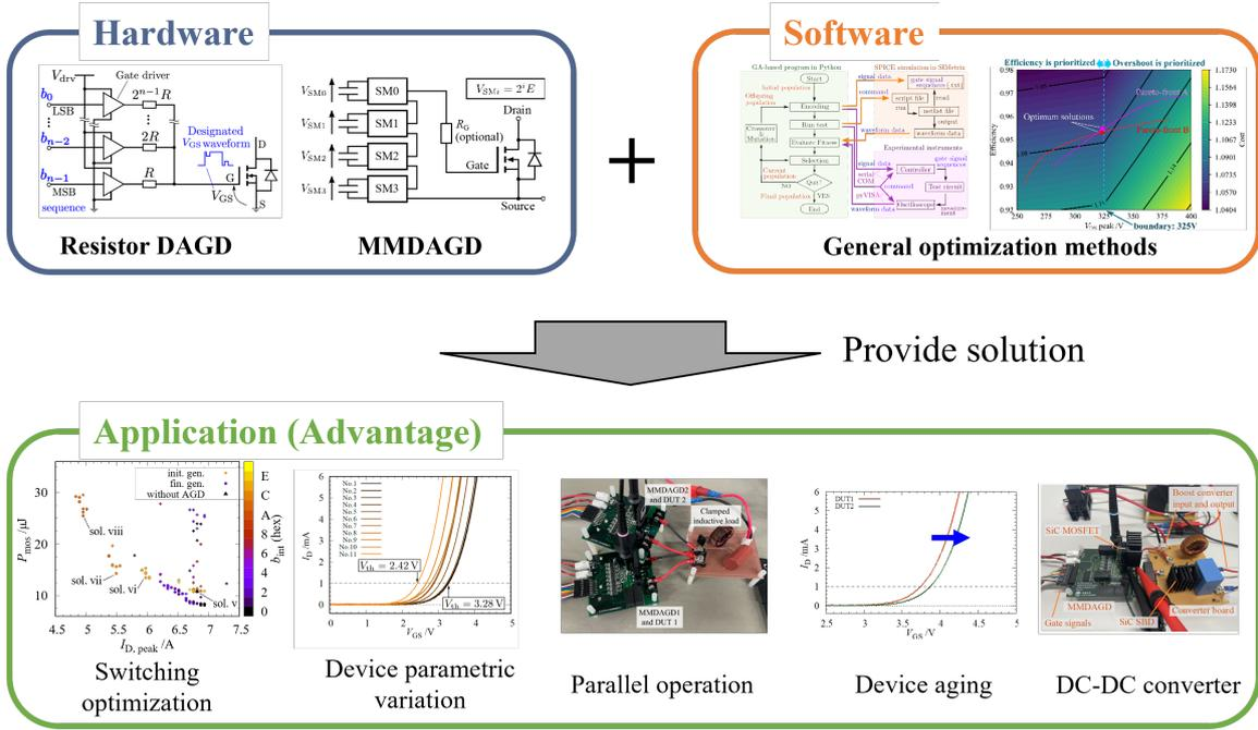
Figure 6.1: Visualization of developed digital active gate drive system.
