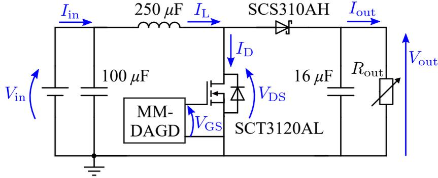
Figure 5.5: Schematic configuration of boost converter. MMDAGD is installed to drive the main SiC MOSFET.
