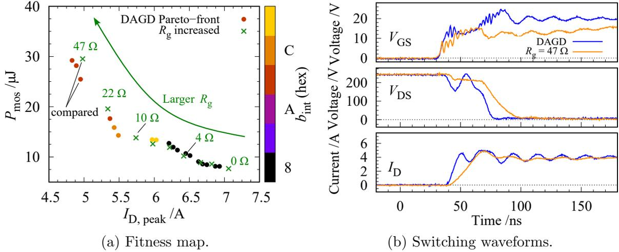
Figure 3.12: Comparison of switching characteristics at turn-on between DAGD (Pareto-front solutions) and standard gate driving with large  $R_G$ .
