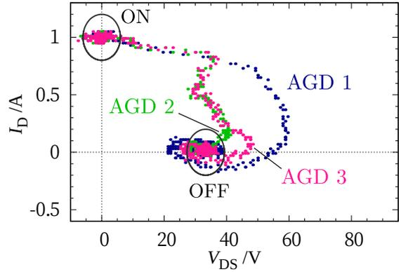
Figure 2.9: Switching trajectories in AGD 1, 2, and 3.
