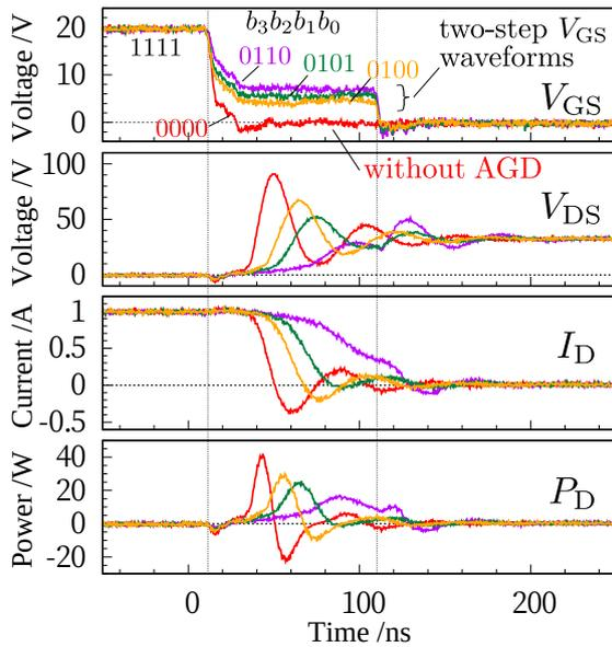
Figure 2.6: Switching waveforms without AGD and with simple two-step  $V_{GS}$  waveforms.
