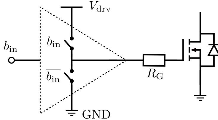
Figure 1.2: Basic configuration of gate drive circuit for power MOSFET.  $b_{in}$  denotes the input logic signal,  $V_{drv}$  denotes the positive DC voltage required to drive the MOSFET, and  $R_G$  denotes the external gate resistor.
