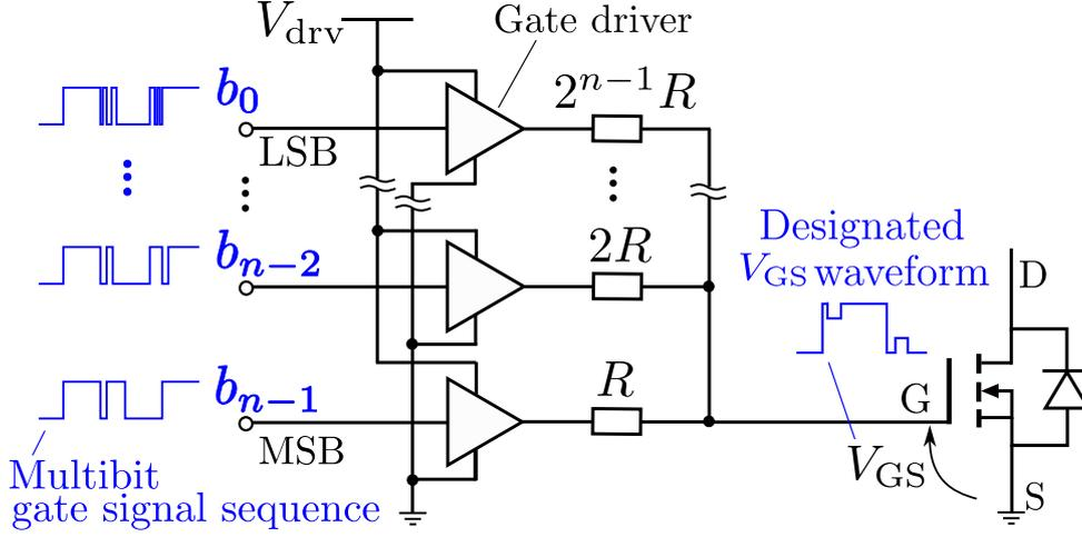
Figure 2.1: Configuration of  $n$ -bit digital active gate driver.
