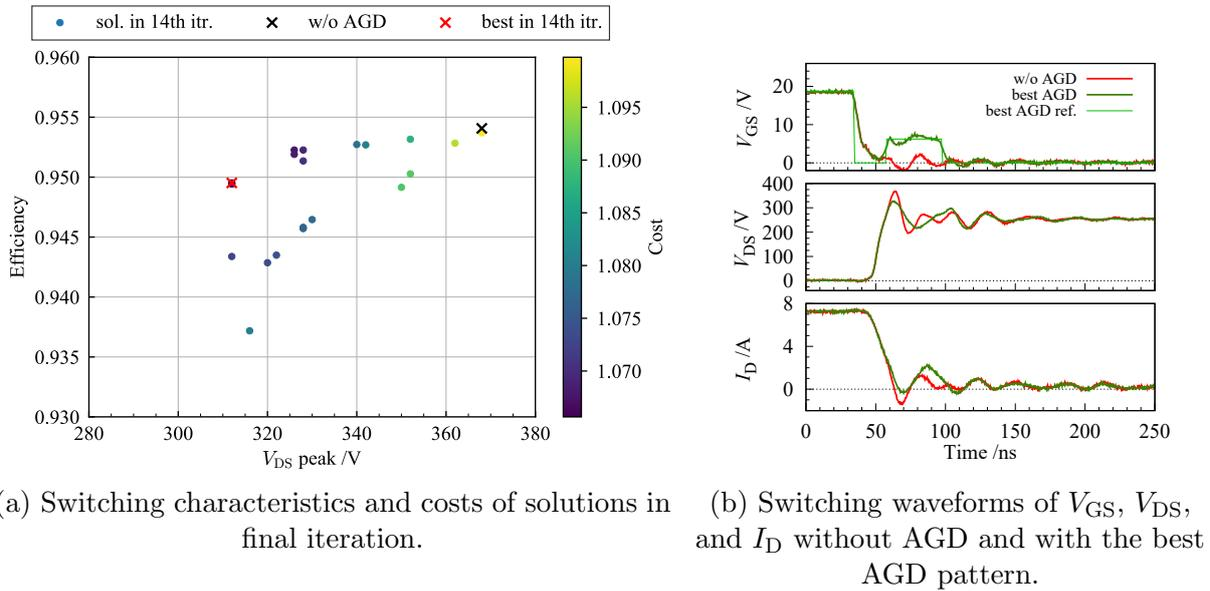
Figure 5.7: Results of initial optimization at turn-off ( $V_{DSbound} = 320$  V).
