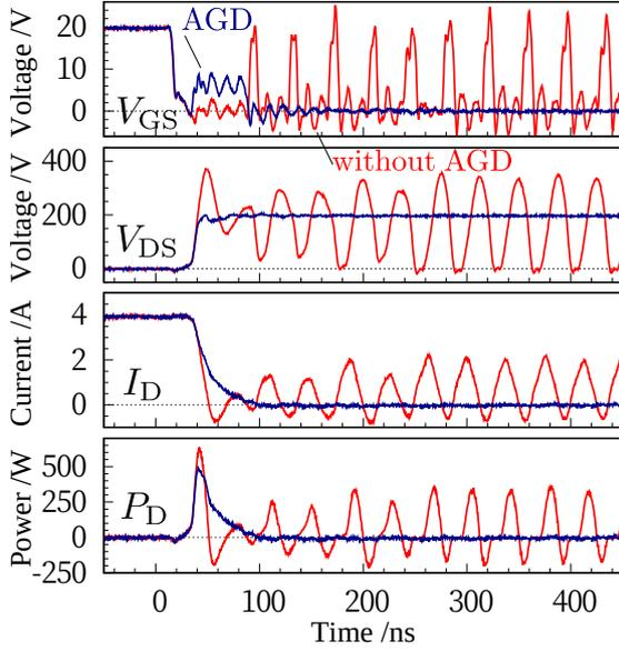
Figure 2.10: Switching waveforms without/with AGD under a higher-voltage condition.
