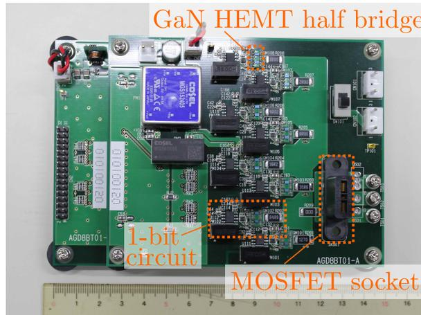
Figure 2.15: Photograph of GaN-HEMT-based 8-bit DAGD.
