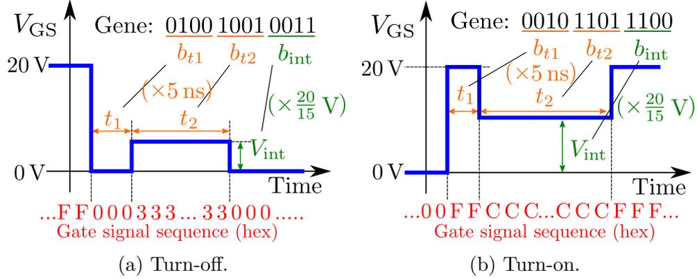
Figure 3.2: Genotype and phenotype of gate signal sequences and corresponding  $V_{GS}$  waveforms. © 2023 IEEE.
