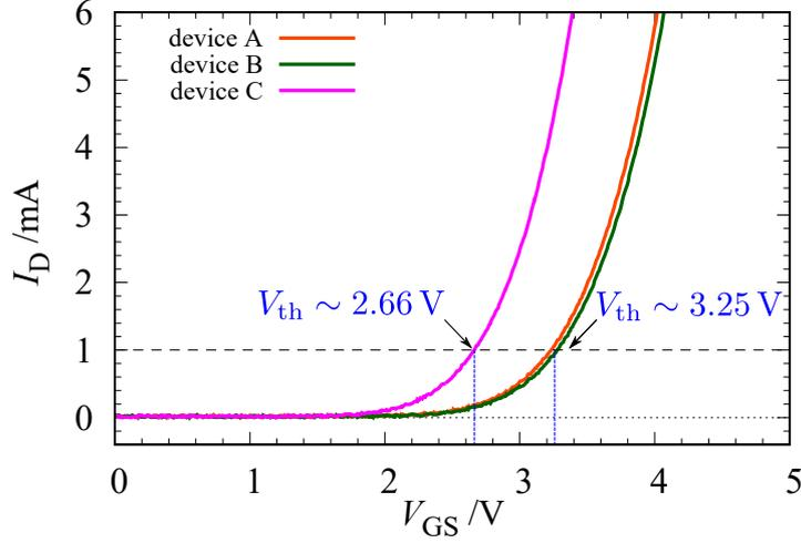
Figure 4.6:  $I_D$ - $V_{GS}$  characteristics and  $V_{th}$  (at  $I_D = 1$  mA) of selected DUTs measured at  $V_{DS} = 10$  V.
