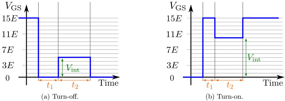
Figure 5.1: AGD patterns using three parameters.
