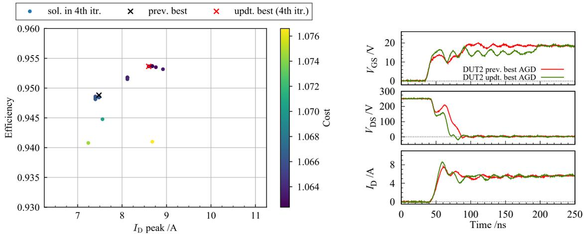
(a) Switching characteristics and costs of solutions in final iteration.
