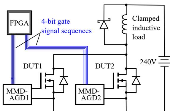
Figure 4.4: Schematic diagram of double-pulse switching test circuit with two parallel-connected SiC MOSFETs. © 2023 IEEE.
