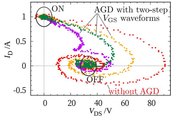
Figure 2.7: Switching trajectories without AGD and with simple two-step  $V_{GS}$  waveforms.
