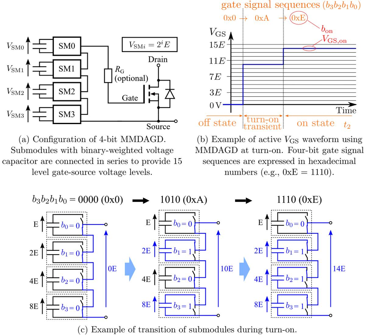
Figure 4.1: Concept and operation of 4-bit MMDAGD. © 2023 IEEE.
