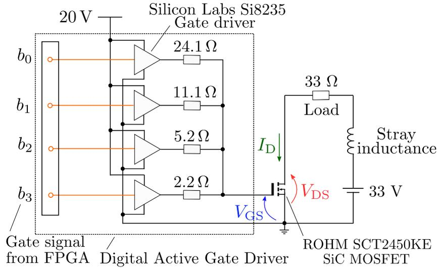
Figure 2.5: Schematic diagram of experimental circuit.
