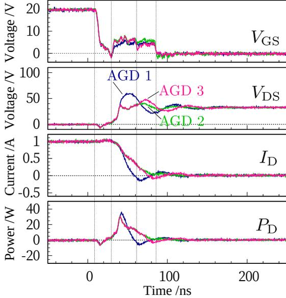
Figure 2.8: Switching waveforms in AGD 1, 2, and 3.
