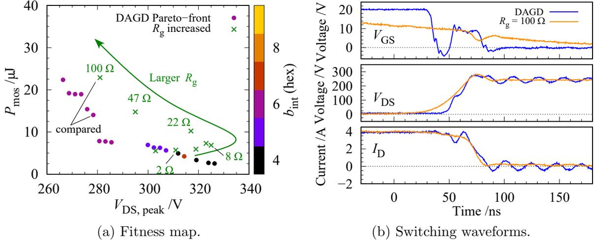
Figure 3.11: Comparison of switching characteristics at turn-off between DAGD (Pareto-front solutions) and standard gate driving with large  $R_G$ .
