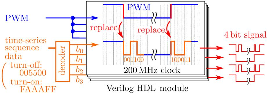
Figure 3.8: 4-bit gate signal generation inside FPGA. © 2023 IEEE.
