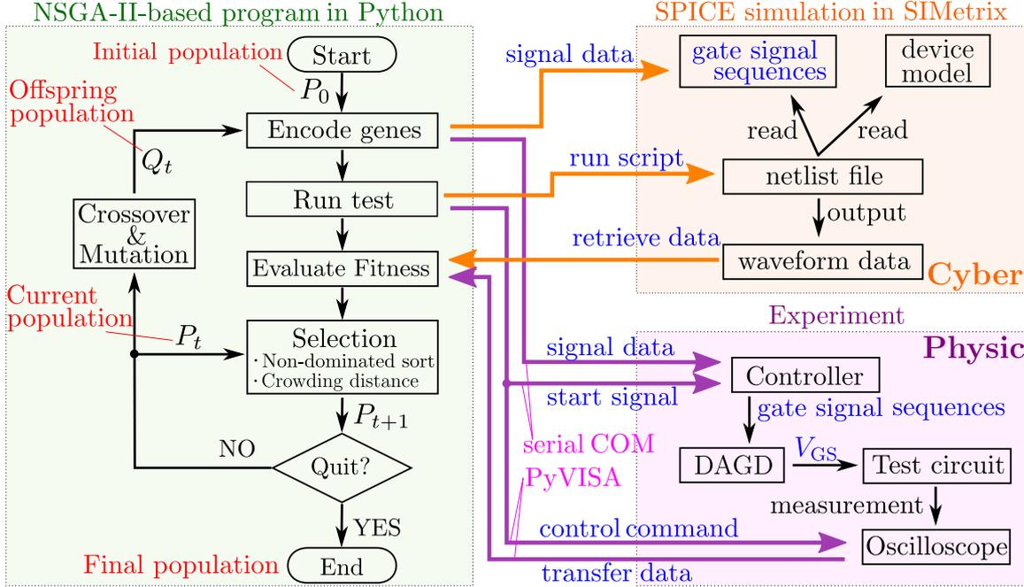
Figure 3.3: Flowchart of optimization process interfacing SPICE simulation (orange area) and experiment (purple area). Orange and purple arrows denotes the data or command transfer between the program in PC and simulation soft/experimental apparatus. © 2023 IEEE.
