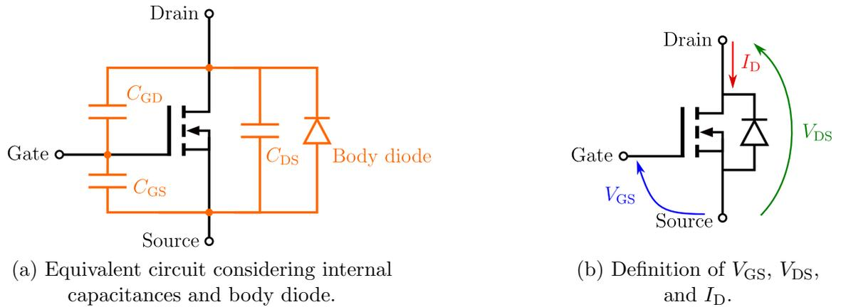
Figure 1.1: Schematic representation of MOSFET.
