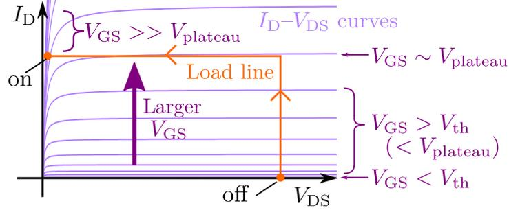
Figure 3.1: Example of  $I_D$ - $V_{DS}$  (drain current vs drain-source voltage) curves of MOSFET and load curve. © 2023 IEEE.
