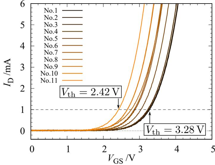
Figure 1.5:  $I_D$ - $V_{GS}$  characteristics of several SiC MOSFETs of the same model measured at  $V_{DS} = 10$  V and at room temperature. Measurement was done using a semiconductor curve tracer (custom-made product, IWATSU Electric Co, Ltd.).  $V_{th}$  is defined here as  $V_{GS}$  level at which  $I_D$  reaches 1.0 mA.
