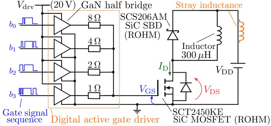
Figure 3.4: Schematic diagram of GaN-HEMT-based 4-bit DAGD and double-pulse test circuit. © 2023 IEEE.
