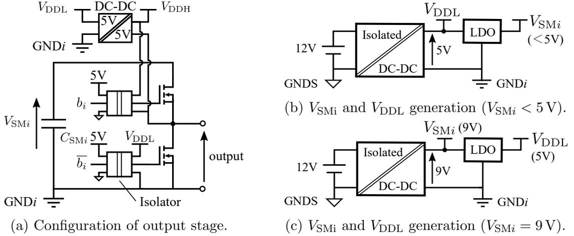
Figure 4.2: Schematic configuration of submodules ( $SM_i$ ) © 2023 IEEE.
