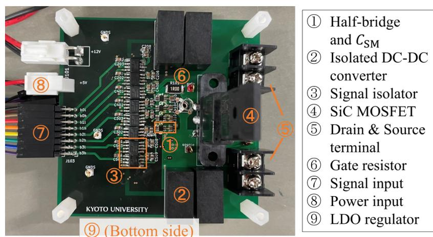
Figure 4.3: Photograph of prototype MMDAGD. © 2023 IEEE.
