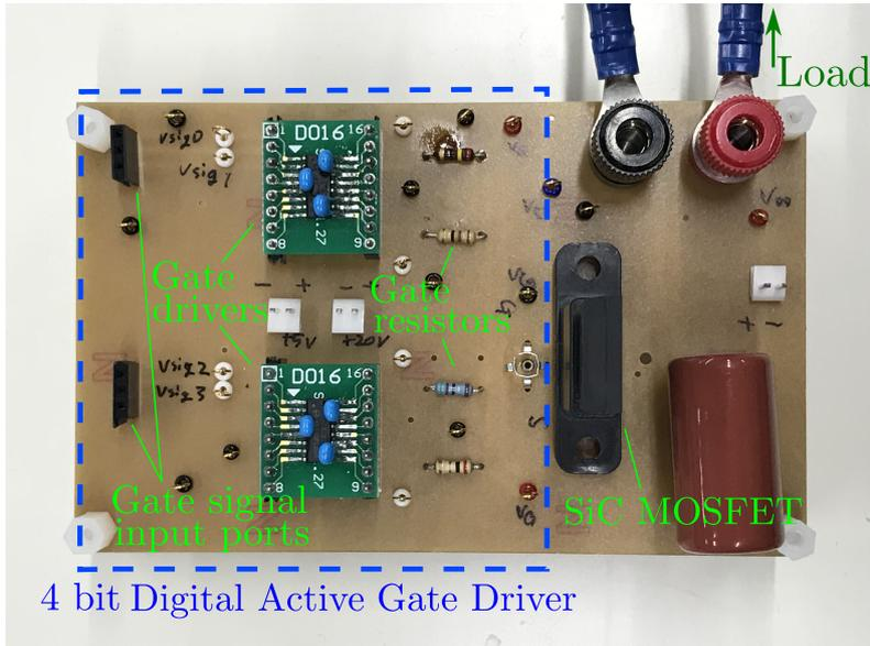
Figure 2.4: Photograph of fabricated circuit.
