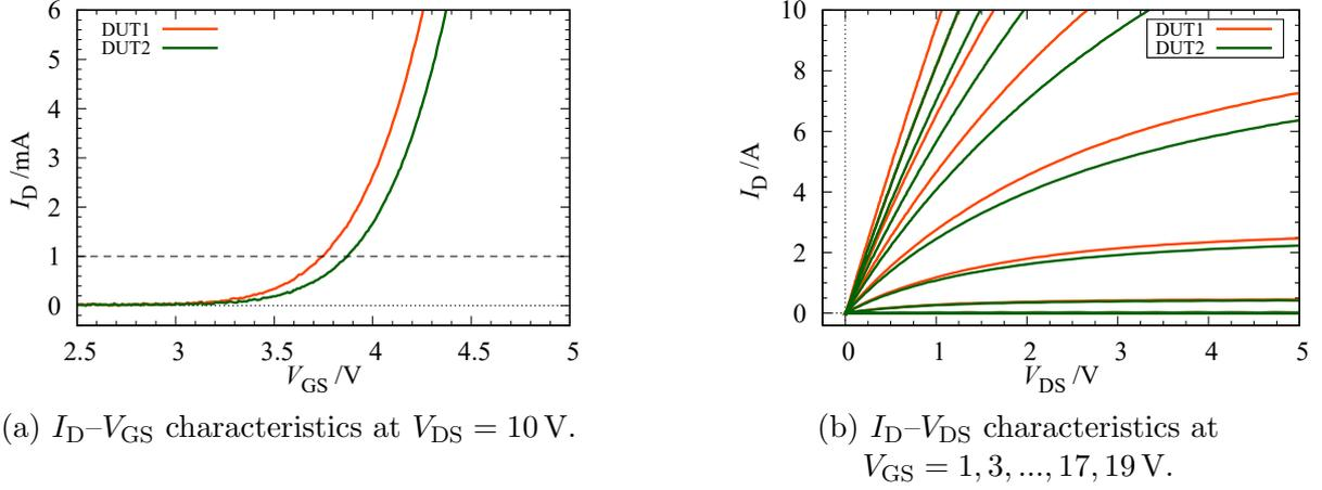
Figure 5.9: Measured device characteristics of the two DUTs.
