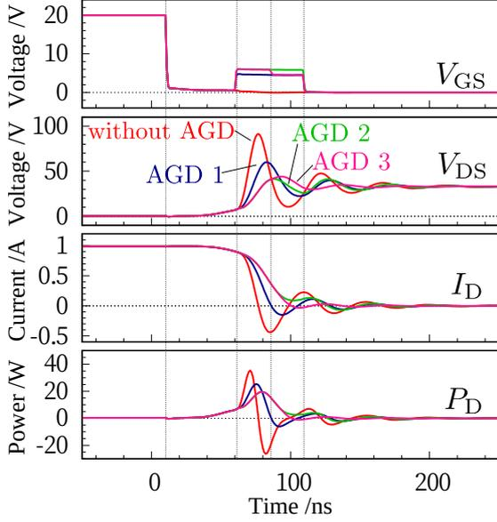
Figure 2.12: Simulated switching waveforms without/with AGD.
