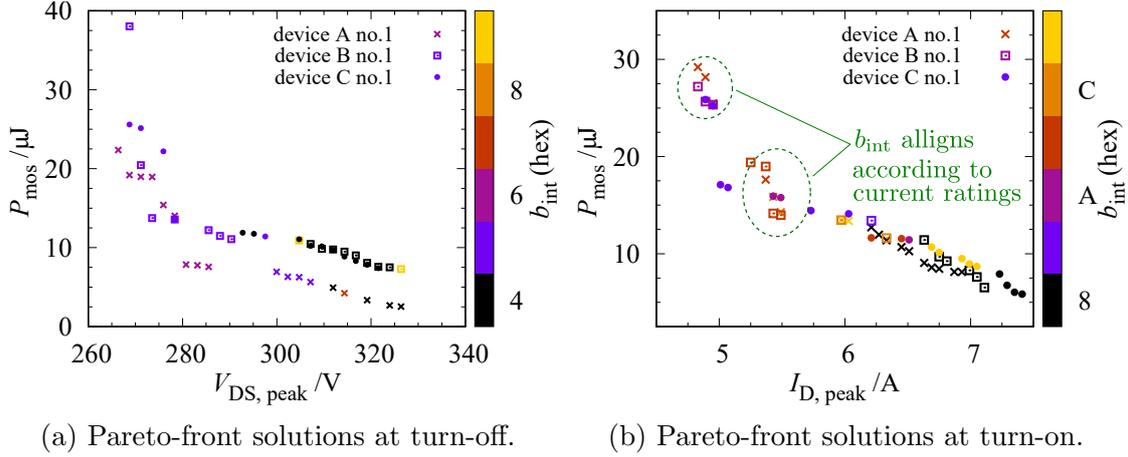
Figure 3.16: Optimization results for SiC MOSFETs with different current ratings.
