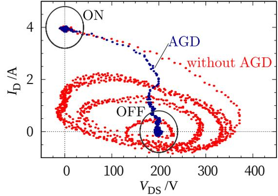
Figure 2.11: Switching trajectories without/with AGD under a higher-voltage condition.
