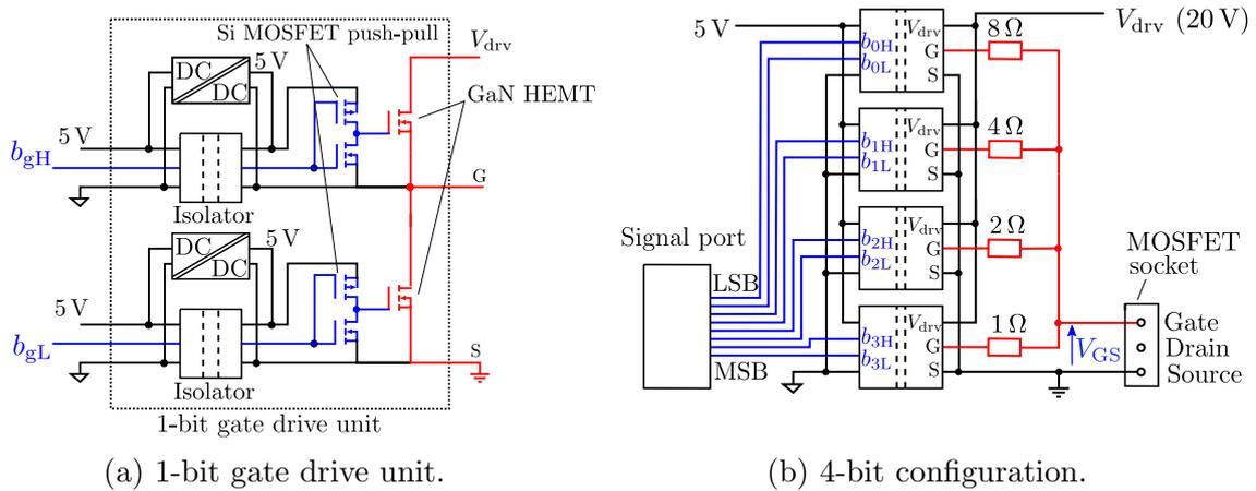
Figure 2.16: Schematic configuration of GaN-HEMT-based digital active gate driver.
