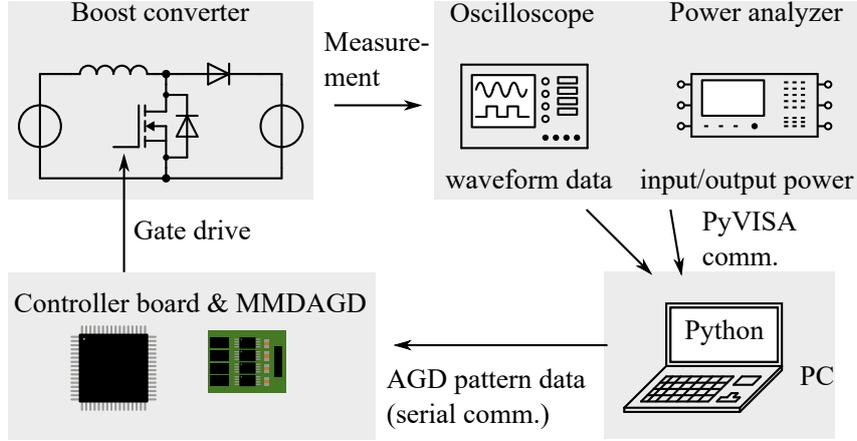
Figure 5.4: Illustration of optimization process in the experiment.
