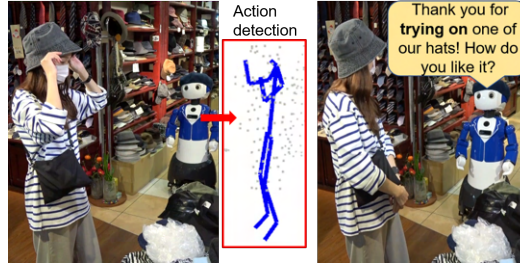
Figure 5.1: The shopworker robot detects the customer’s action and starts to encourage them.
