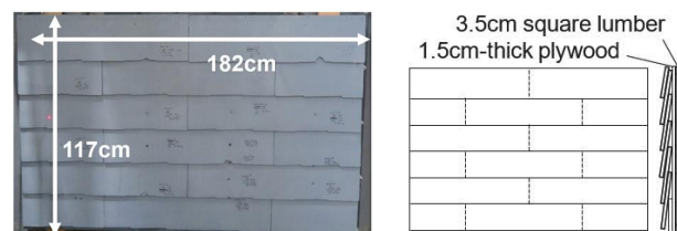
Fig. 6. Slate Tiles Roofing. Slate tile: Knew Colonial, Base material: lauan plywood, 12 mm-thick.
