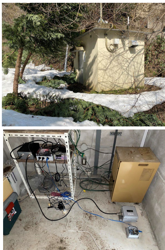
Photo 2 : Status of test observations at the DP.HRJ observation hut. (Upper) The appearance of the observation hut. (Bottom) Inside the observation hut. ADXL355 and JEP-8A3 are bonded to the concrete floor at the lower right.
