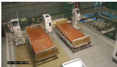
(A) Base-isolated (PFA = 92  $\text{cm/s}^2$ , PFV = 17  $\text{cm/s}$ )
