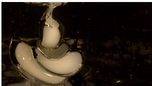
Photo 6 An example of dry-ice bubbles observed when dry-ice is put into water
