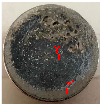
(a) Platinum foil-brazed surface with carbon coating
