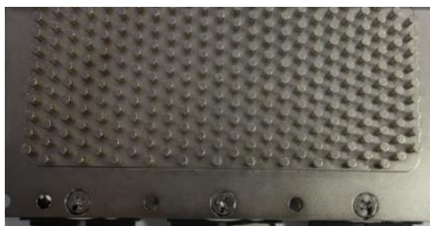
Figure 1-7. Water cooling heatsink (Nickel plated copper pin fins)
