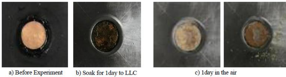
Figure 1-24. Images of heating surface before/after LLC boiling experiment. (a)Before experiment, (b)Soak for 1 day to LLC and (c)1 day in the air. [49]
