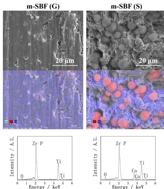
Figure 1. The SEM images, EDX mappings, and EDX spectra of Zr-50Ti alloys pretreated with or without sulfuric acid solution and then soaked in m-SBF. The “m-SBF (G)” signifies grinding-only Zr-50Ti alloys soaked in m-SBF for 1 day, and the “m-SBF (S)” signifies sulfuric acid-treated Zr-50Ti alloys soaked in m-SBF for 1 day.
