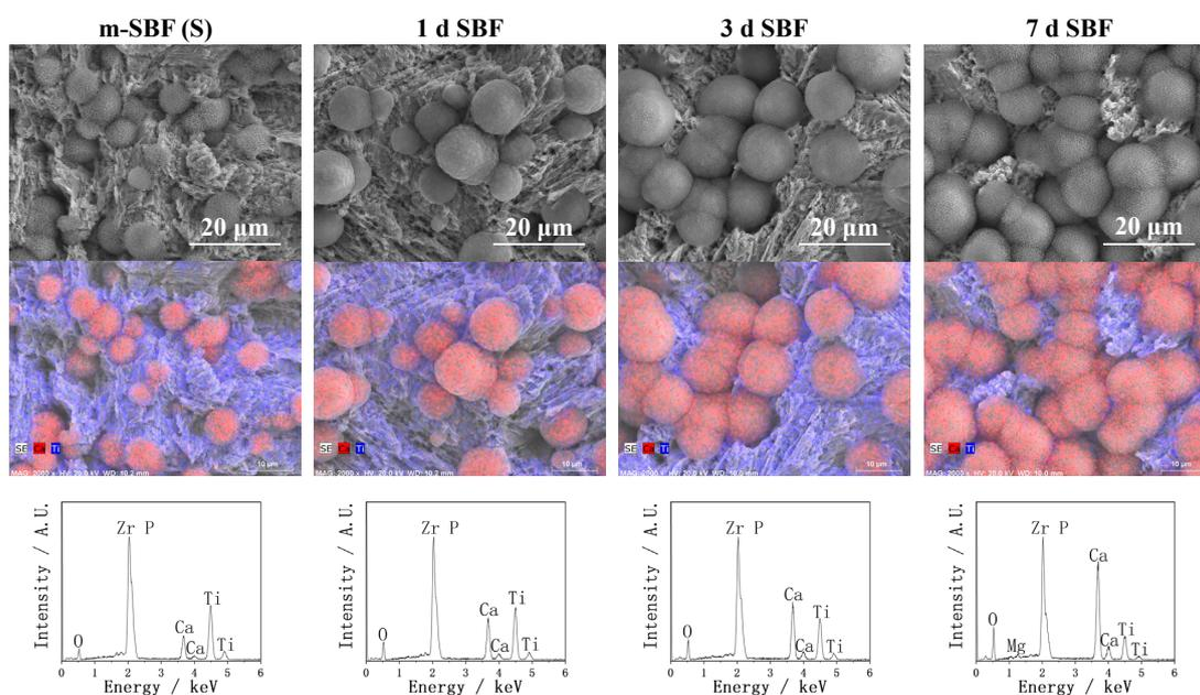
Figure 2. The SEM images, EDX mappings, and EDX spectra of sulfuric acid-treated Zr-50Ti alloys subsequently soaked in m-SBF and then soaked in SBF. The “m-SBF (S)” signifies sulfuric acid-treated Zr-50Ti alloys soaked in m-SBF for 1 day, the “1 d SBF”, “3 d SBF”, and “7 d SBF” signifies acid-treated Zr-50Ti alloys soaked in m-SBF for 1 day and then soaked in SBF for 1, 3, and 7 days, respectively.
