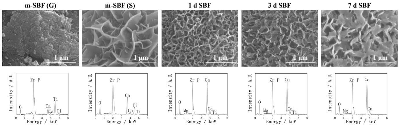
Figure 3. The SEM images and EDX spectra of Zr-50Ti alloys magnified from the center point of the corresponding place in Fig. 1 and Fig. 2. The “m-SBF (G)” signifies ground-only Zr-50Ti alloys soaked in m-SBF for 1 day, the “m-SBF (S)” signifies sulfuric acid-treated Zr-50Ti alloys soaked in m-SBF for 1 day, the “1 d SBF”, “3 d SBF”, and “7 d SBF” signifies acid-treated Zr-50Ti alloys soaked in m-SBF for 1 day and then soaked in SBF for 1, 3, and 7 days, respectively.
