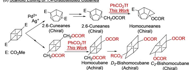
**Figure 1.** (a) A use of homocubanes as phenoxy bioisostere. (b) Scaffold editing strategy of 1,4-disubstituted cubanes into other hexahedrons by  $\text{PhCO}_2\text{Tf}$  catalyst.
