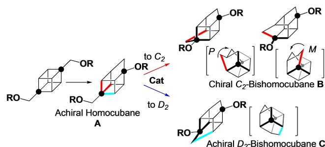
**Scheme 3.** Formation of  $C_2$ -(**B**) and  $D_2$ -homocubanes **C** via sequential rearrangements from 1,4-bis(acyloxymethyl)cubane using *in situ* prepared catalyst.
