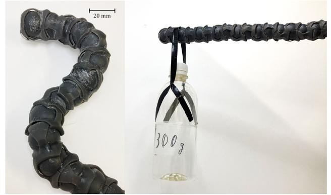
**FIGURE 6.** Prototype of the spherical-layer-type unit with a single layer. The prototype is fixed in a rod-like shape, lifting a 300 g weight.
