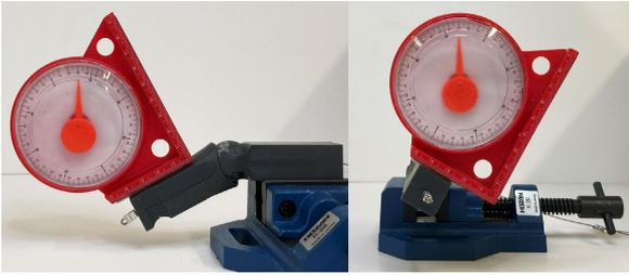
**FIGURE 7.** Measurement of the motion range of the spherical-layer type unit. Left:  $y, z$  axes, right:  $x$  axis.
