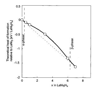
FIG. 4. Theoretical heat of formation of six models as a function of H content, x, relative to the energy of LaNi<sub>5</sub>. The phase boundaries correspond to averaged experimental values in many reports. Note that they were not determined by the calculation.
