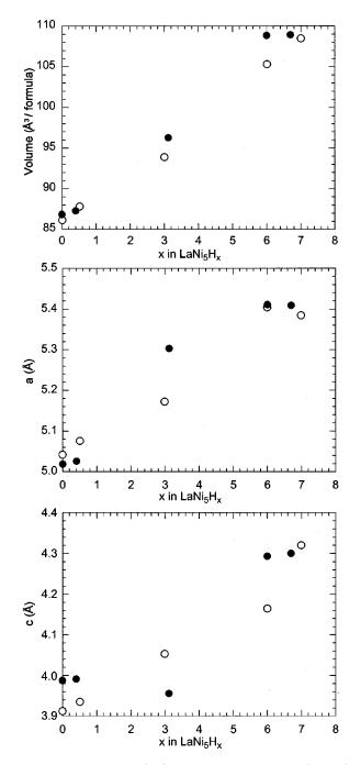
FIG. 5. Comparison of (top) volume, lattice constants (middle) a and (bottom) c between calculated (open circles) and experimental (closed circles) (Refs. 4,27,30,42) for composition, x.
