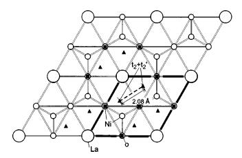
FIG. 2. The array of atoms projected on the (0001) plane for Model  $3^*$  of LaNi<sub>5</sub>H<sub>7</sub>. The thick lines make a unit cell.
