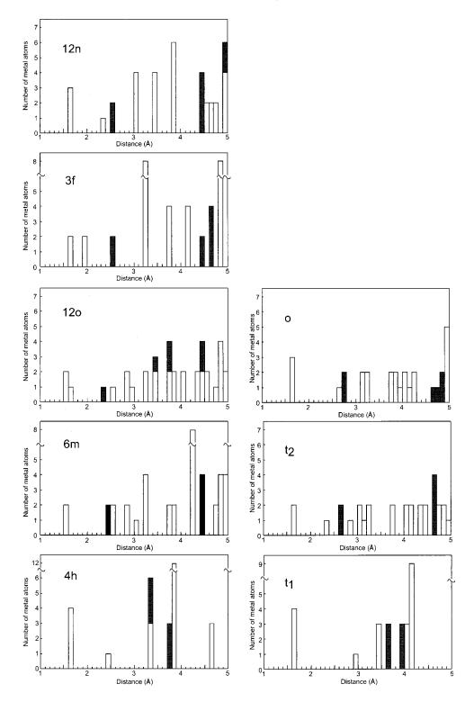
FIG. 3. Radial distribution of near-neighbor La or Ni atoms around a H atom at the interstice. Left: The models for primary solid solutions,  $LaNi_5H_{0.5}$ . Right: The model for  $LaNi_5H_7$ (Model 1\*).
