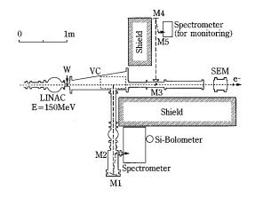
FIG. 1. The arrangement of the experiment. (VC) a vacuum chamber; (W) a titanium window 15  $\mu$ m thick; (M2, M3, M5) plane mirrors; (M4) a spherical mirror; (SEM) a secondary emission monitor; and ( $e^{-}$ ) electron beam.
