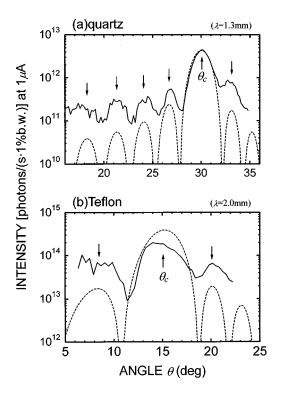
FIG. 5. The angular distribution of radiation from the quartz of 60 mm long at  $\lambda = 1.3$  mm and the teflon of 100 mm long at  $\lambda = 2.0$  mm. The data are plotted on a logarithmic scale in order to visualize satellite peaks in the angular distribution.
