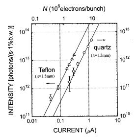
FIG. 6. The relation between the intensity and the beam current. The solid lines represent quadratic dependence of P on N.
