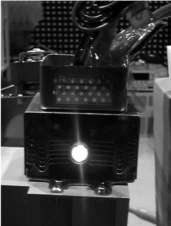
Fig. 4. Photo of the magnetron for the measurements of the filament temperature. The light of the filament is seen through a crystal plate.
