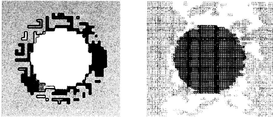
The left figure shows a form of the bone obtained by the computation and the right figure depicts a horizontal section of bone structure supporting a cylindrical dental implant.
