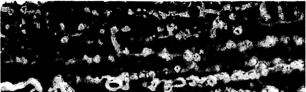
Fig. 3. Pattern of parallel vortex filaments comprising a series of the loop solitons, generated by the XeCl excimer laser ( E = 250 J; t = 16 ns), on Co-coated steel surface. The length L of the filaments is about 500 \mu\text{m} , and the core size is d \sim 5 - 7 \mu\text{m} . The horizontal and vertical dimensions of the picture are 1,100 \mu\text{m} and 300 \mu\text{m} .
