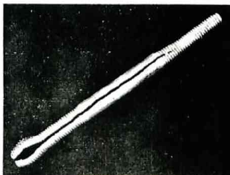
Photo. 4 Steel pipe burst by the detonation (6.0 and 1.6 mm in outer and inner diameters respectively.)
