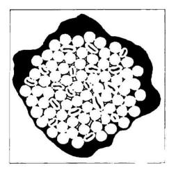
Warp yarn can be sized with starch. Or with Poval, our water soluble polyvinyl alcohol.
