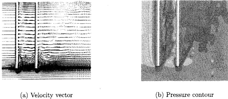
Figure 2: Computational results on the x-z plane across circular cylinders
