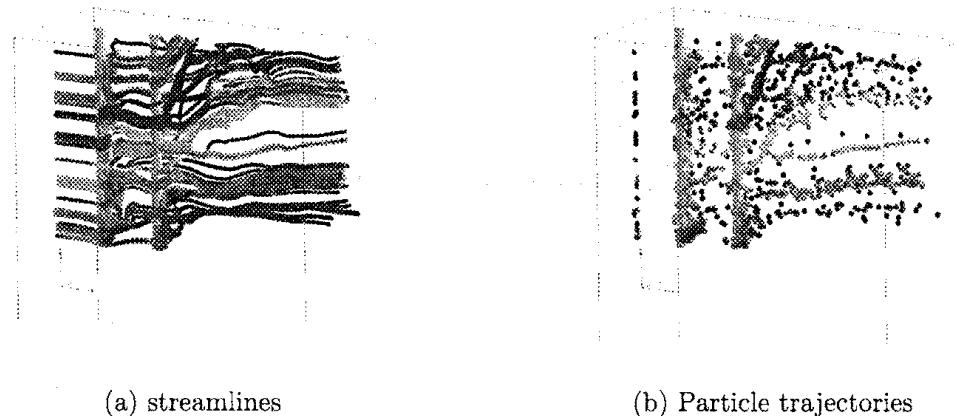
Figure 3: Upward flow motions observed behind two circular cylinders
