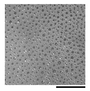
Confocal transmission microscopy image of the oil/water interface 15 hours after its preparation. Phospholipid is DOPC (0.1 mol% NBD-PC) at a concentration of 0.8 mM in oil. Spontaneously emulsified water-in-oil droplets, visible as dark circles, arranged at the interface into regular arrays, in agreement with previous observations reported in the literature<sup>[11]</sup>.
