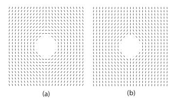
FIG. 4. Nematic director n for (a)  $\lambda_e/R=10$  and (b) 4.2 at  $\varepsilon_1/\varepsilon_0=-1$  in the xz plane. A pair of point defects can be seen in (a), while there is no defect in (b).
