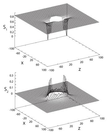
FIG. 6. Scalar order parameter  $S_1$  and biaxiality parameter  $S_2$  for  $\lambda_e/R=10$  and  $\varepsilon_1/\varepsilon_0=-1$  in the xz plane. They deviate from the background values around the disclination line segments.
