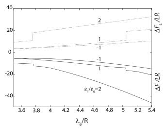
FIG. 10. Normalized changes of the total free energy Eq. (4.7) (solid lines) and the Landau–de Gennes free energy Eq. (4.6) (broken lines) vs  $\lambda_e/R$  for three  $\varepsilon_1/\varepsilon_0$ . For  $\varepsilon_1>0$  the discontinuities correspond to the defect formation in Fig. 9.
