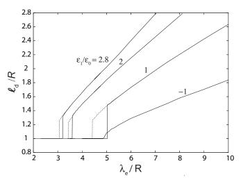
FIG. 9. Normalized defect radius  $\ell_d/R$  vs  $\lambda_e/R$  for various  $\varepsilon_1/\varepsilon_0$ . For positive  $\varepsilon_1$  the defect formation and collapse are discontinuous, where the solid and dotted curves are the results of increasing and decreasing  $\lambda_e$ , respectively. For negative  $\varepsilon_1$  the transition is continuous with a critical point.
