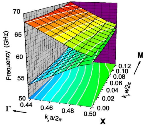
FIG. 9. (Color online) Detailed dispersion around X point drawn in two-dimensional wave number plane. Collisionless plasma column has a diameter of 1.0 mm in a square lattice with lattice constant of 2.5 mm and the electron density was  $10^{13} \text{ cm}^{-3}$ .
