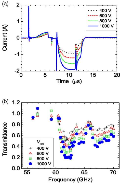
FIG. 4. (Color online) (a) Time evolutions of discharge currents for various applied monopolar voltage  $V_{dc}$ . (b) Frequency dependence of transmittance signals of millimeter waves in TE mode as a function of  $V_{dc}$ . Discharge gas was He at 200 Torr,  $V_{ac}=900V_{0p}$ , and the row number of plasma columns is 30.
