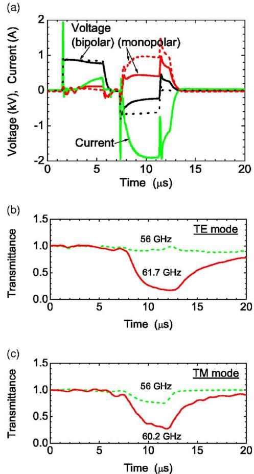
FIG. 3. (Color online) (a) Time evolutions of applied and discharge voltages and discharge currents. Solid and dotted lines in voltage indicate signals at supply output and on electrode, respectively. (b) Transmittance signal of millimeter waves in TE mode. (c) Transmittance signal of millimeter waves in TM mode.
