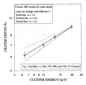
FIG. 3. Crater depth calculated by molecular dynamics for  $Ar_n$  (n = 236, 370, 490, and 736) cluster ion impact with energy of 27 eV/atom on a Cu(100) surface (circles), the straight line corresponds to the  $E^{1/3}$  power law. For comparison, the power-law dependencies with the exponents  $\alpha = 0.4$  (dotted line) and 0.25 (dashed line) are also given.
