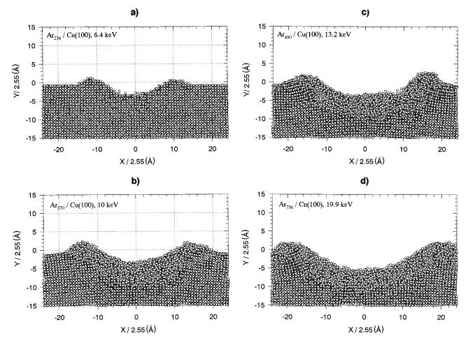
FIG. 5. Side view of the craters formed on a Cu(100) surface calculated by MD for  $Ar_n$  (n = 236, 370, 490, and 736) cluster ion impact, at 6.4 keV after 17 ps (a), and 10 keV (b), 13.2 keV (c), 19.9 keV (d) after 6 ps from the beginning of an impact.
