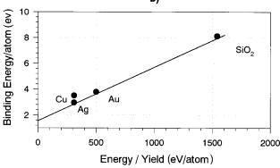
FIG. 7. Brinell hardness data from available literature are correlated linearly to energy per sputtered atom (yield) (a), and binding energy data are correlated with the energy per yield (b). The binding energy for SiO<sub>2</sub> 8.12 eV is taken from Ref. 37.
