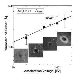
FIG. 6. Energy dependence of the crater diameters obtained by STM (images of the craters are given below each data point) at  $Ar_{3000}$  cluster ion impacts, with total energy of 20-150 keV, on a Au (111) thin film surface deposited on mica (Refs. 21, 22). The straight line in this figure represents the  $\frac{1}{3}$  dependence of crater diameters on the acceleration voltage.
