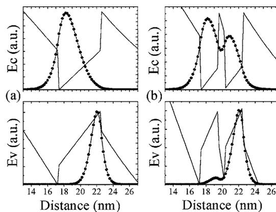
FIG. 1. Energy band profile and wave function of (a) 5-nm-thick In<sub>0.16</sub>Ga<sub>0.84</sub>N SQW and (b) In<sub>0.16</sub>Ga<sub>0.84</sub>N (2 nm)–Al<sub>0.05</sub>Ga<sub>0.95</sub>N (1 nm  $\delta$  layer)–In<sub>0.16</sub>Ga<sub>0.84</sub>N (2 nm) QW sandwiched between 10-nm-thick GaN barriers under zero bias current.
