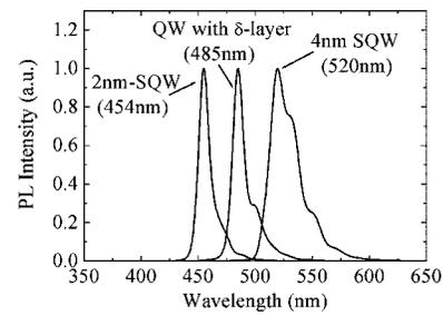
FIG. 3. Low-temperature (13 K) cw PL spectra of nominally undoped 2-nm-thick  $\text{In}_{0.16}\text{Ga}_{0.84}\text{N}$  SQW,  $\text{In}_{0.16}\text{Ga}_{0.84}\text{N}$  (2 nm)- $\text{Al}_{0.05}\text{Ga}_{0.95}\text{N}$  (1 nm)- $\text{In}_{0.16}\text{Ga}_{0.84}\text{N}$  (2 nm) QW, and 4-nm-thick  $\text{In}_{0.16}\text{Ga}_{0.84}\text{N}$  SQW.
