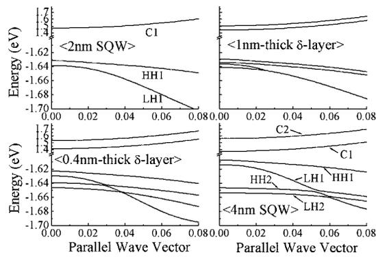
FIG. 2. The in-plane dispersion of conduction and valence subbands of 2-nm-thick  $\text{In}_{0.16}\text{Ga}_{0.84}\text{N}$  SQW,  $\text{In}_{0.16}\text{Ga}_{0.84}\text{N}$  QW with embedded 4-Å- and 10-Å-thick  $\text{Al}_{0.05}\text{Ga}_{0.95}\text{N}$   $\delta$  layers, and 4-nm-thick  $\text{In}_{0.16}\text{Ga}_{0.84}\text{N}$  SQW.
