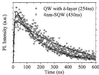
FIG. 5. Low-temperature (13 K) PL decay dynamics of the 4-nm-thick SQW and the QW structure with the  $\delta$  layer around the PL peak wavelength of 520 nm.
