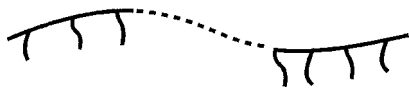
FIG. 1. Schematic sketch of the model molecule, [(-\text{CH}_2\text{CH}_2)_4(-\text{CH}_2\text{CH}(\text{C}_6\text{H}_{13})-)(-\text{CH}_2\text{CH}_2)_5]_{50} . The main chain is 500-mer polyethylene. The number of ends is 52.
